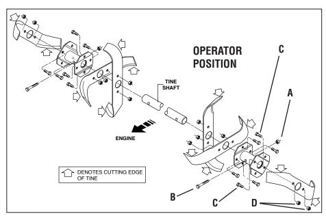
Figure 5-3: Tines, tine holders and installation hardware.
